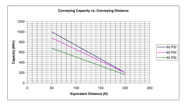
Equivalent distance calculated using the following: 1' horizontal pipe = 1' equivalent distance 1' vertical pipe = 2' equivalent distance 90° pipe bend = 10' equivalent distance 1' hose = 4' equivalent distance 35#/ft<sup>3</sup> material Standard unit represents 50' equivalent distance 200' equivalent distance was 90' horizontal pipe, 20' material hose and 3 90° pipe bends
